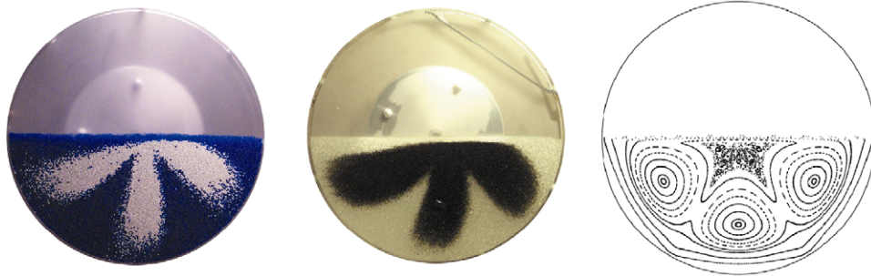
Fig. 2. Radial segregation of bidisperse granular materials (S-systems in dry and slurry states) in periodically forced tumblers. The system is half full and has a forcing frequency of 6 cycles/revolution. Left image is the dry system, middle image is the same system in a slurry state, and the right image is the corresponding Poincaré section made using a continuum model (Fiedor and Ottino, 2005).
