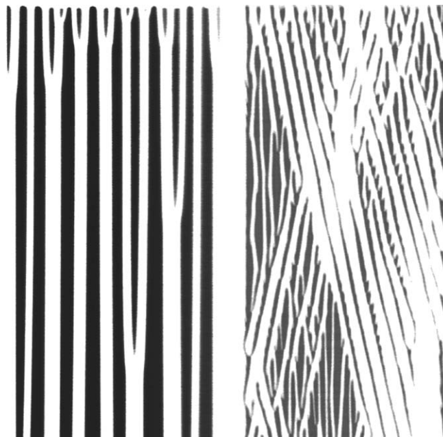
Fig. 1. Axial segregation of bidisperse S-systems in dry and slurry states. Left: Axial segregation in slurries; the rotation rate is 3 rpm; Right: Axial segregation and traveling waves in a dry system at a fast rotation rate (25 rpm) (from Fiedor and Ottino, 2003).
